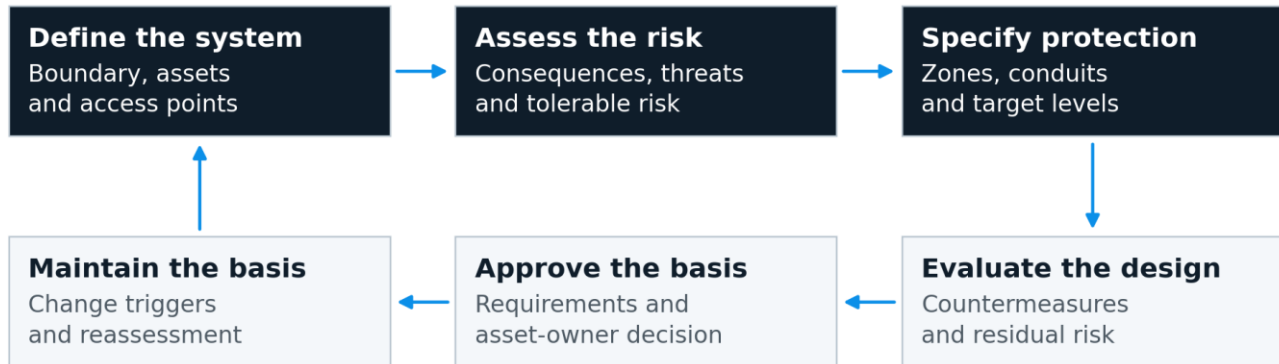
Figure 2. Simplified engineering interpretation of the part 3-2 workflow. Risk assessment and zoning are iterative; this is not a reproduction of the normative process.
